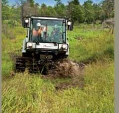
PRINOTH's vehicles are made like no other and the Trooper's combination of strength, agility and versatility will exceed your expectations at every turn. Powered by an EPA Euromot-compliant Cate pillar turbo diesel engine with 142 horsepowe (106 Kw) and 556 N·m of torque (410 lb·ft) the Trooper packs a tight punch. Multiple tract options and a footprint lighter than your own only 48 g/cm² (0.68 psi), means you can take the Trooper over extreme terrain in any season
