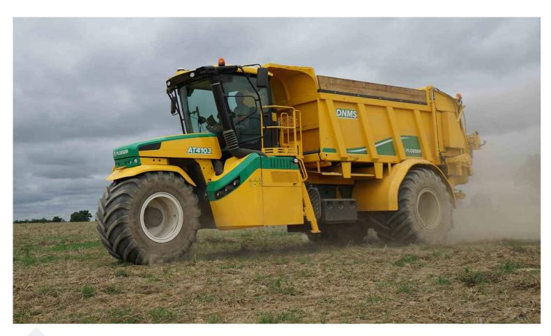
The AT4103 DNMS has a **Tebbe spreader** superstructure with a wide bin (internal width 2.56 metres). The wear-resistant bin and wear parts are made from Hardox steel. The metering valve height can be adjusted hydraulically. The compost is transported by the Rübig bottom conveyor belt to the two horizontal beaters and two metering discs with a diameter of 1.20 metres. The speed of the separately driven beaters and metering discs can be regulated from 300 to 800 rpm.
