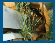
Loading versatility: Load to the left, right, or rear, the choice is yours! A full 180 degrees of rotation on the conveyor makes harvest quick and easy.
