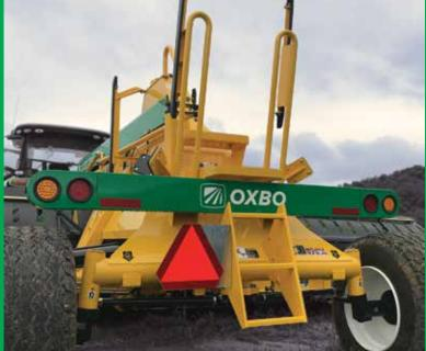
**NEW!** Rear mounted hydraulic tank and access platform make hydraulic system maintenance easier
